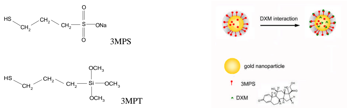
Figure 1: Thiols used for the AuNPs functionalization: 3MPS and interaction scheme of AuNPs with DXM
